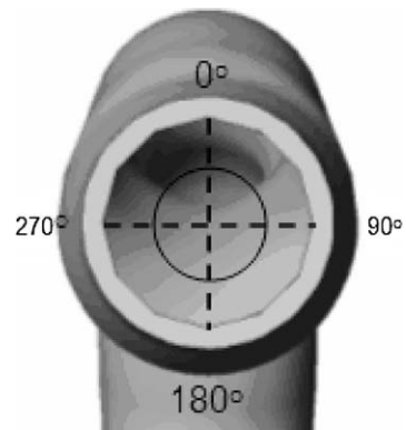
Fig. 4. Injection angles and 40% radius circle for oral airway experiments, looking into the mouth of the oral airway.
